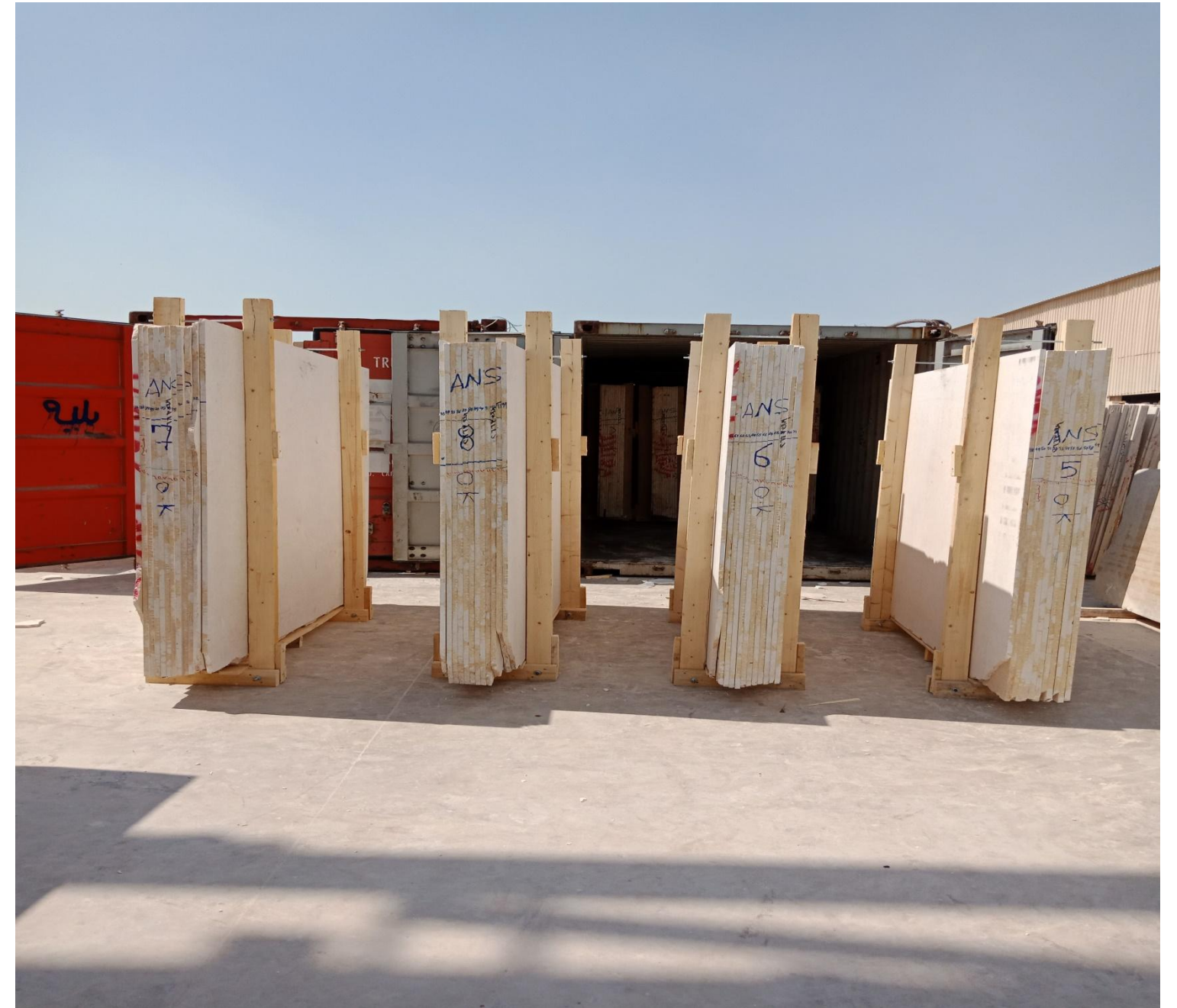
Wooden Bundles For slabs
